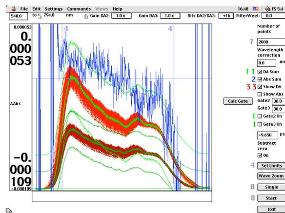
9) Diode array diagnostics 1: Averaged intensity & gate levels; 2: Averaged absorption; 3: All 2000 individual intensities; 4: Limits for scaling of  $\Delta$ Abs; 5: Wavelength range; 6,7,8: See fig 8
