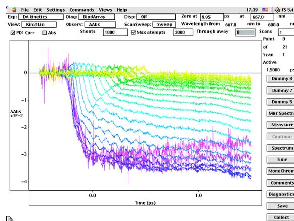
15) Kinetic traces of a single sweep, 5 seconds accumulation time including the back sweep.
