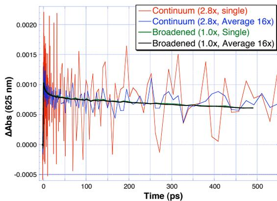
20) Single diode channel traces for Trp excited at 295 nm. Average of 16 adjacent diode channels.
