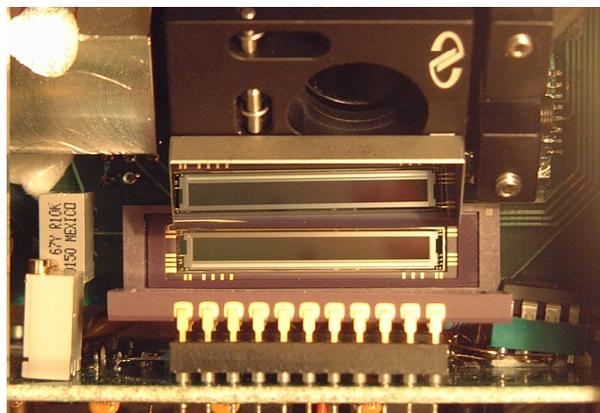
13) Diode array detection head for a small spectrograph.
