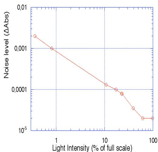
7) Noise level for the diode array versus probe light intensity after averaging 1000 times.
