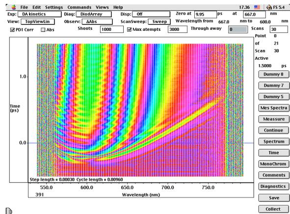
19) Top view with colour coded amplitudes. One cycle through the spectrum represent 9.6 mAbs. Sweep data averaged 30 times.
