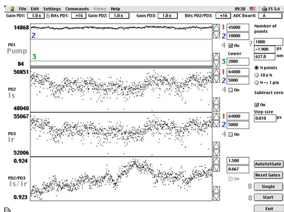
8) PDs vs time diagnostics. 1: Upper gate level; 2: Lower gate level; 3: Chopped pump gate level; 4: Gate on/off; 6: Digitizer options; 7: Number of collected points; 8: Collect single or repetitive.
