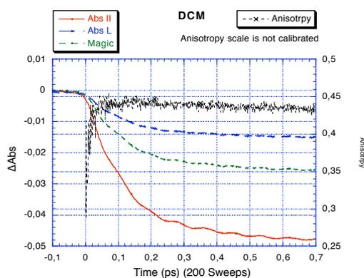
2) *Single wavelength anisotropy kinetics. Both parallel and perpendicular polarisations are collected simultaneously.*
