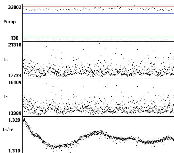
6) The intensities of 1000 consecutive laser pulses (200 in case of the pump, so that the chopping is clearly seen). The coloured lines are gate levels
