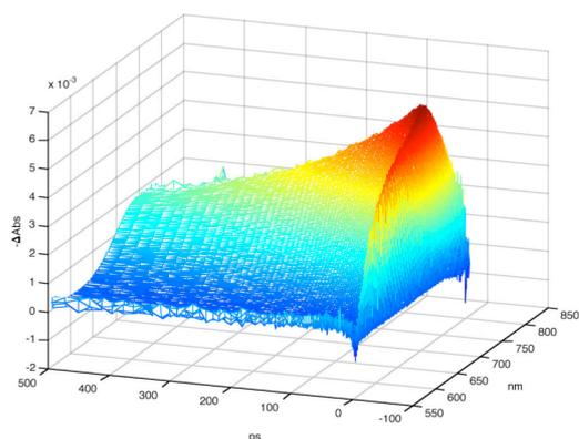
1) *Multiwavelength absorption kinetics: the diode array collects a whole spectrum for each laser shot.*
